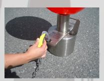
• The carbine hook on one end of the chain is hooked into the hole in the spreader wing of the device.
