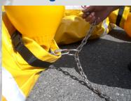
The supplied 6 mm stainless steel chain is run through the rings which are attached to the neck fitting of each dummy.
