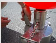
The chain end is inserted into the chain lock on the device base and is locked in place as the cocking lever is released.
