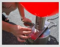
• The spring loaded locking mechanism is cocked open using the lever on the side.
