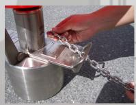
The free end of the chain is run through the steel guide on the opposite spreader wing.
