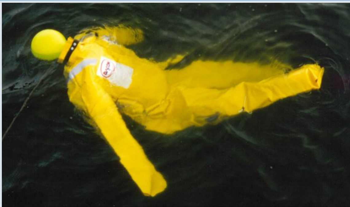
Dacon Rescue Dummy - adjusted for horizontal floating position
