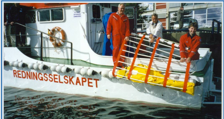
Recovery of the Dacon Rescue Dummy using the Dacon Rescue Frame
