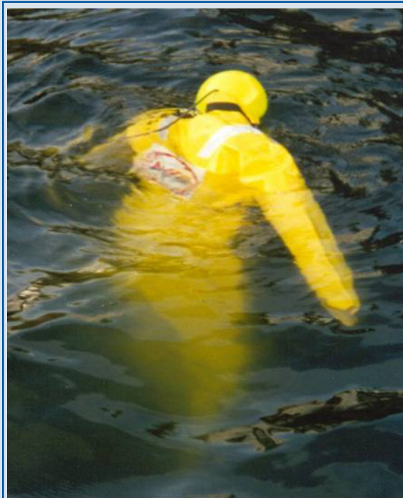
Dacon Rescue Dummy - adjusted for vertical floating position
