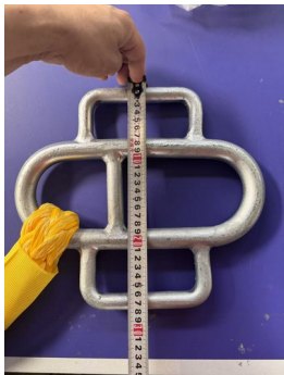
Fig. 5 — Overall length of connector plate: ± 260 mm
