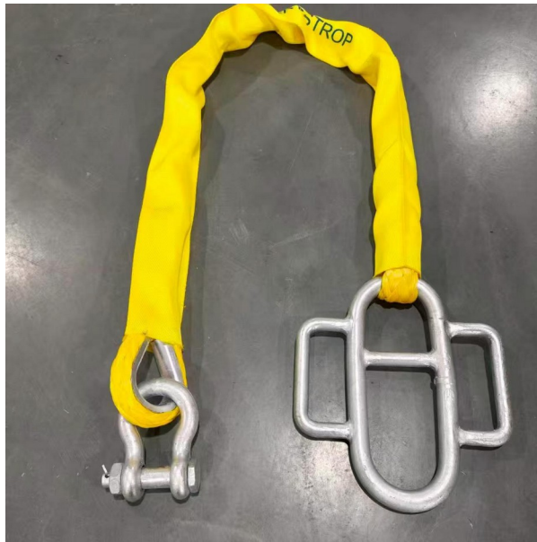
Fig. 1 — Complete recovery strop: webbing sling, forged connector plate and bow shackle
